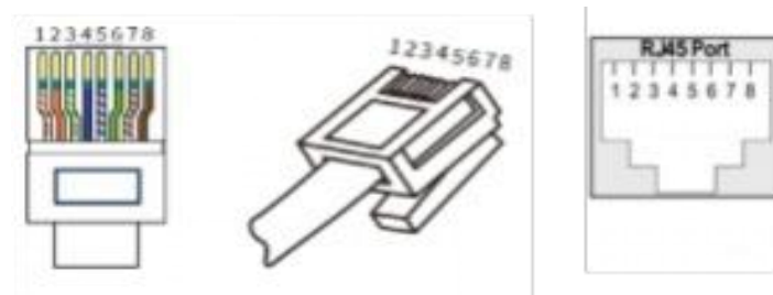
Figure 2-8 “Inverter CAN/RS485” port pins
